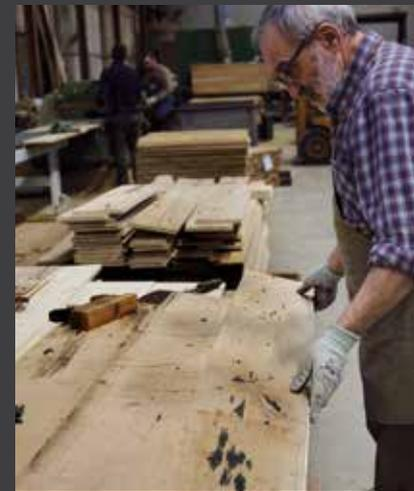
For this reason we carefully follow every stage of production. First we prepare the briccole for the subsequent phases with attentive removal of extraneous elements and by careful washing. We then proceed to the cutting of the poles so as to obtain axes of various lengths and thicknesses, suitable for the realization of different products. Having made the cut we can start the drying procedure, moment of prime importance in the entire production process:
